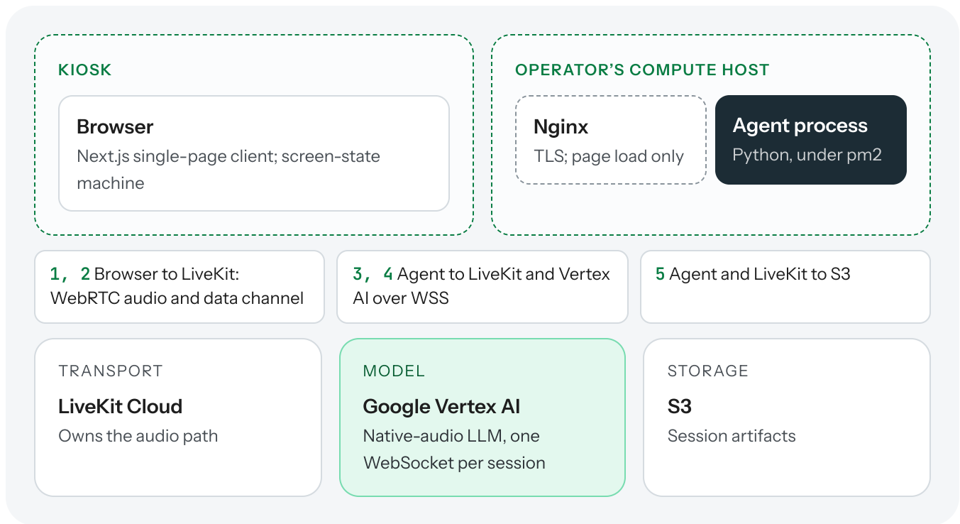
Figure 2. The self-contained kiosk stack. Wire numbers refer to Section 3.3.
