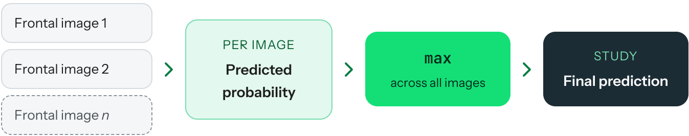
Figure 6. Test-time aggregation: the study-level prediction is the maximum predicted probability across all frontal images linked to the study.
