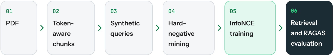
Figure 4. The synthetic-supervision pipeline for LoRA fine-tuning of Qwen3-Embedding-8B.
